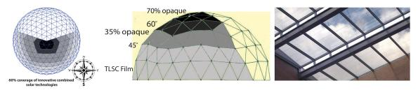
Thin Layer Solar Collection (TLSC) film is used from the base of the dome up to 45° and is totally transparent because it only interacts with UV and Infared light, letting the visible wavelengths pass through. The film directs theses wavelengths to the edge of the panel where the solar cells are located.
